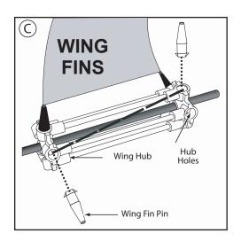
PLEASE NOTE: If you make a mistake in the placement of the Wing Fins (i.e. backward, wrong color sequence etc.), you can remove them by carefully inserting a small flat end screwdriver between the base of the Wing Fin Pin and the hub and pushing it up and out.
