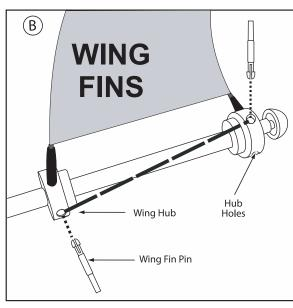
PLEASE NOTE: If you make a mistake in the placement of the Wing Fins (i.e. backward, wrong color sequence etc.), you can remove them by carefully inserting a small flat end screwdriver between the base of the Wing Fin Pin and the hub and pushing it up and out.
