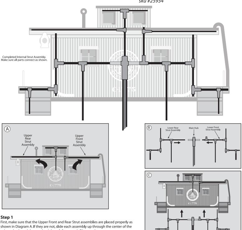
shown in Diagram A. If they are not, slide each assembly up through the center of the spinner body and then to the right or left to match Diagram A.
