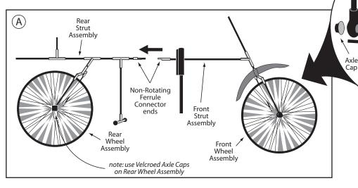
Spinner Step 2 Slide Axle Rod into center tube of Spinner Wheel. Slide rubber ends of Fork on Front Strut Assembly over ends of Axle Rod. Pound Non-Velcroed Axle Caps onto ends of Axle Rod using a hammer or some other blunt instrument. Repeat for Rear Strut Assembly using Velcroed Axle Caps. (inset, diagram A)
