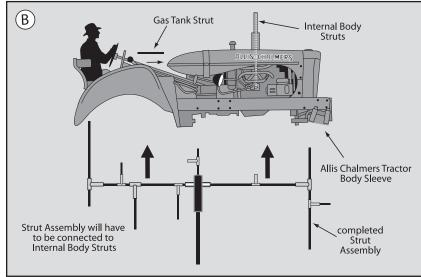
The Strut Assembly of your Allis Chalmers Tractor spinner is shipped in three sections. Connect Center Rods of the Rear Strut Assembly and the Front Strut Assembly to the Center Rod of the Center Strut Assembly as shown. (diagram A)
