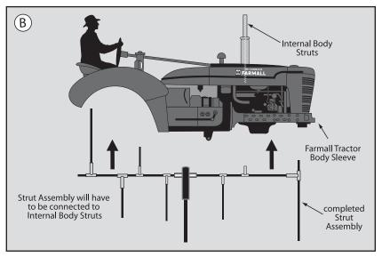
Step 1 The Strut Assembly of your Farmall Tractor spinner is shipped in three sections. Connect Center Rods of the Rear Strut Assembly and the Front Strut Assembly to the Center Rod of the Center Strut Assembly as shown. (diagram A)
