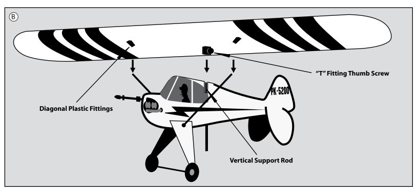
**Step 2**Slide the wing "T" Fitting Thumb Screw onto the Internal Vertical Support Rod. Then insert the Landing Gear Struts into the two black Diagonal Plastic Fittings on either side of the wing. Be sure to tighten the Wing "T" Fitting Thumb Screw to secure the wing to the fuselage. Make sure the wing is fully seated on the Vertical Support Rod. (diagram B)
