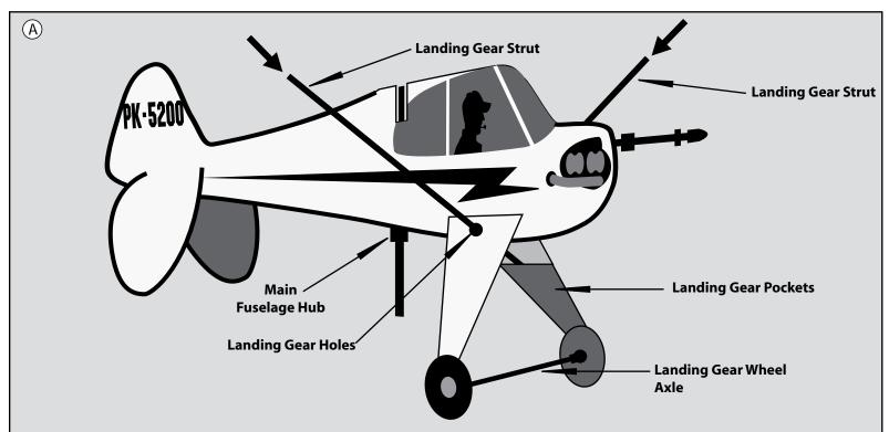
**Step 1**Insert both Landing Gear Struts through the Landing Gear Holes into the Landing Gear Pockets, located at the front of the plane. These struts should cross each other and form an "X". Then insert the Landing Gear Wheel Axle into the two black fittings located between the two Landing Gear Pockets. (diagram A)
