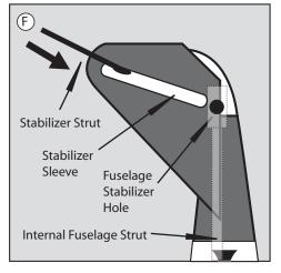
Internal Wing Strut into the Aluminum Ferrule, which is inside the square channel of the Main Fuselage Hub. Secure the wings to the fuselage with the Velcro tabs on both the top and bottom of the Left and Right Wings. (diagram C & D)
