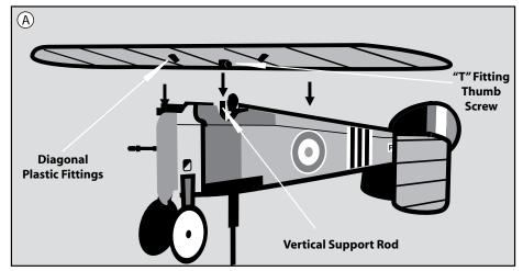
Slide the top wing's "T" Fitting Thumb Screw onto the Internal Vertical Support Rod. Be sure to tighten the top wing's "T" Fitting Thumb Screw to secure the wing to the fuselage. Make sure the wing is fully seated on the Vertical Support Rod. (diagram A)
