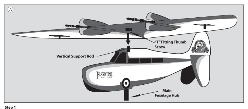
Slide the wing "T" Fitting Thumb Screw onto the Internal Vertical Support Rod. Be sure to tighten the Wing "T" Fitting Thumb Screw to secure the wing to the fuselage. Make sure the wing is fully seated on the Vertical Support Rod. Make sure the engine cowlings are perpendicular to the wing. (diagram A)
