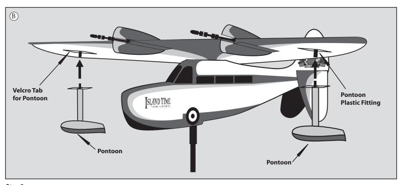
**Step 2**Insert the Pontoon struts into the two plastic fittings on wither side of the wing. Secure the Pontoons onto the under side of the wing with the Velcro tabs. (diagram B)
