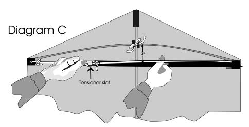
3. Before flying, cross struts must be bowed approximately 7" by tensioning the Bow Strings.
